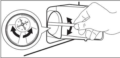
10. Replace the filter into the pump by inserting it correctly into the special guides. Screw the pump cover firmly by turning it clockwise.
