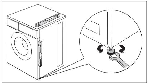
Some vibration is inevitable, especially if mounted on a wooden floor. Sprung wooden floors are particularly susceptible to vibration. For advice, consult a builder. If possible, always place the machine on a solid floor.
