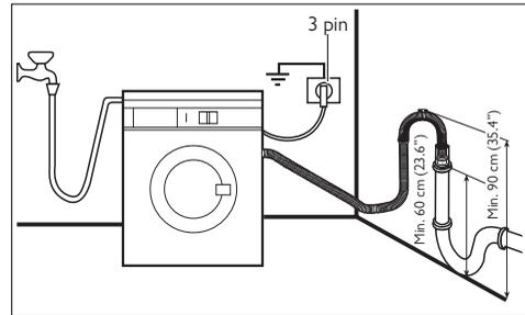
The drain hose may be extended to a maximum of 4 metres. An additional drain hose and joining piece is available from your local Service Force Centre. The joining piece must have an internal diameter of 18 mm. If your drain hose looks like this (see below) you do not require the "U" piece". Just push the hose firmly in to the standpipe.
