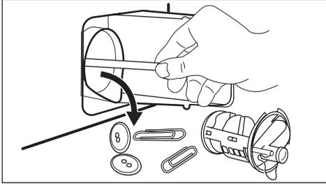
9. Check carefully whether the pump impeller rotates (it rotates jerkily). If it doesn't rotate, please contact your Service Centre.
