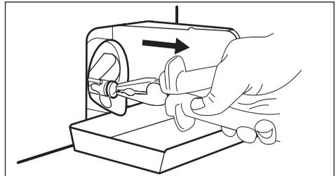
7. When no more water comes out, unscrew the pump cover by turning it anti-clockwise, using pliers, and remove the filter. Always keep a towel nearby to dry up any water spillage when removing the cover. Clean the filter under a tap, to remove any traces of fluff.
