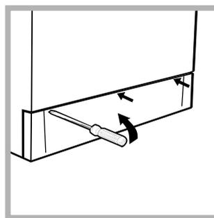
1. using a screwdriver, remove the cover panel on the lower front of the Washer-dryer (see figure);
