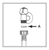
1. Insert seal A into the end of the inlet hose and screw the latter onto a cold water tap with a 3/4 gas threaded mouth (see figure). Before making the connection, allow the water to run freely until it is perfectly clear.
