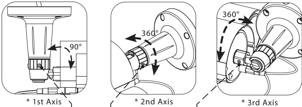
Loosen socket head allen screws to change angle and/or rotate body about base.
