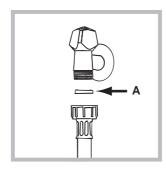
1. Insert seal A into the end of the inlet hose and screw the latter onto a cold water tap with a 3/4 gas threaded mouth (see figure).
