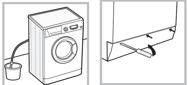
2. make sure the water level inside the machine is lower than the door opening; if it is not, remove excess water using the drain hose, collecting it in a bucket as indicated in the figure.
