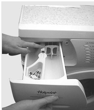
2 Press button to release drawer latch and remove dispenser drawer.
