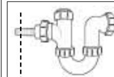
cut off the blocked end of the under sink drainage unit.
