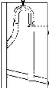
Insert drainage hose approximately 100mm into the standpipe.
