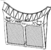
Wash or vacuum clean the filter occasionally. Don't be alarmed by the amount of fluff you may find on the filter. It's part of the wearing, washing and drying process.
