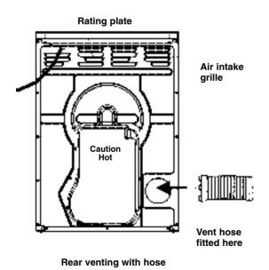
NOTE: When the dryer is in use, avoid touching the back of the machine as it may be hot.
