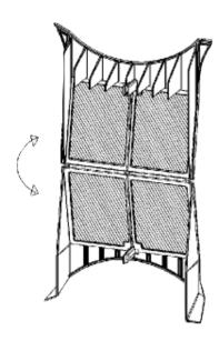
A very important part of your dryer is the fluff filter at the front edge of the drum. It's there to trap the particles of lint and fluff which are normally blown away when clothes are dried on the washing-line.
