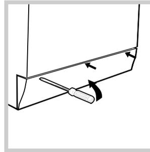
1. Remove the kick strip on the front of the machine using a screwdriver (*see figure*);
