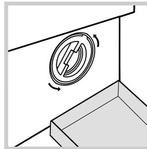
2. Position a container collecting the drained water (approximately 1.5 l) correctly (*see figure*);
