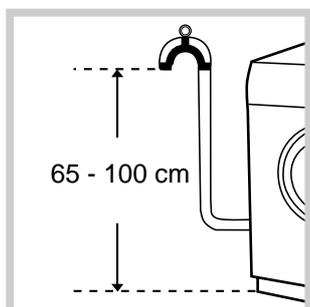
Connect the drain hose, without kinking it, to a draining duct or a stand pipe situated between 65 and 100 cm from the floor;
