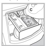
To avoid exceeding the maximum capacity, a buzzer (beep) will sound with growing intensity to signal the level and 3 long beeps will sound once the tank is completely full. Start the wash cycle immediately after filling the tanks to ensure that the dispenser is properly cleaned. The respective icons (for the detergent) and (for the fabric softener) will light up gradually to signal the level.
