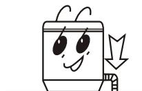
4. Slanting or uneven ground may result in unstable working or abnormal noise. Please make the machine stand horizontally.
