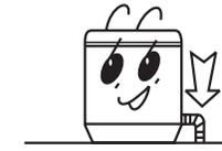
4. Slanting or uneven ground may result in unstable working or abnormal noise. Please make the machine stand horizontally.
