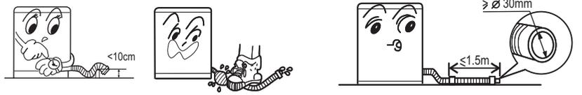
3. If the drain hose is too long, cut it at mid point. To make smooth drainage, cut the front end of the hose slantingly.
