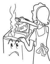
Do not put the machine at damp place like the bathroom. Never wash it with water. Do not put wet laundries on the control panel.
