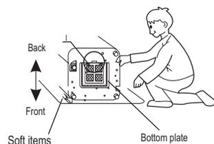
Two claws at the bottom cover shall be inserted in two bar-shaped holes in the stand. Make sure the claws are firmly in place.
