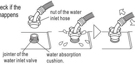
The new hose-sets supplied with the appliance are to be used and that old hose-sets should not be reused.
