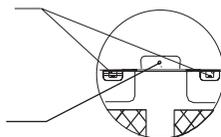
Fasten the bottom plate to base frame with one screw
