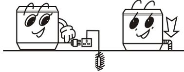
4. Slanting or uneven ground may result in unstable working or abnormal noise. Please make the machine stand horizontally.
