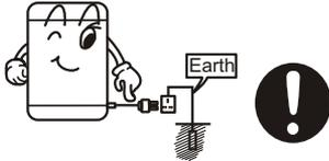
When the machine is normally using, please put the power plug at the location easily to be inserted and extracted by hand. Be sure to pull the plug off when there's power failure, or the machine is being moved, cleaned or when it is idle.
