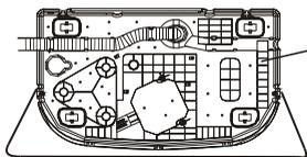
Ventilation hole at the bottom of the washing machine
