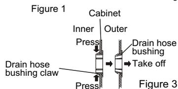
3. Dismantle the protecting cover of the drain outlet at the other side (method the same as the bushing). Install the bushing as per indicated in Figure 4.
