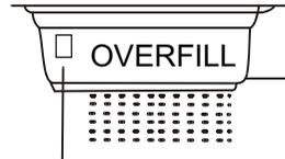
If you find water flowing out here, please twist the water tap to limit the water filling.
