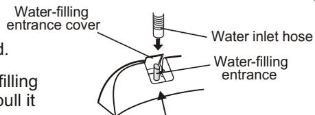
Insert the water inlet hose into the water-filling entrance on the control panel directly. (pull it out to dismantle it)
