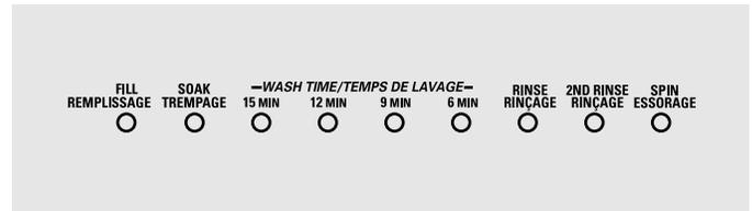
The Cycle Indicator Lights show what stage the washer is in. The wash time is the length of the wash agitation. The **6 MIN** light will remain lit during drain and spin. When the Selector knob is set to a new cycle the Indicator Lights will flash momentarily, showing what stages the cycle will go through.
