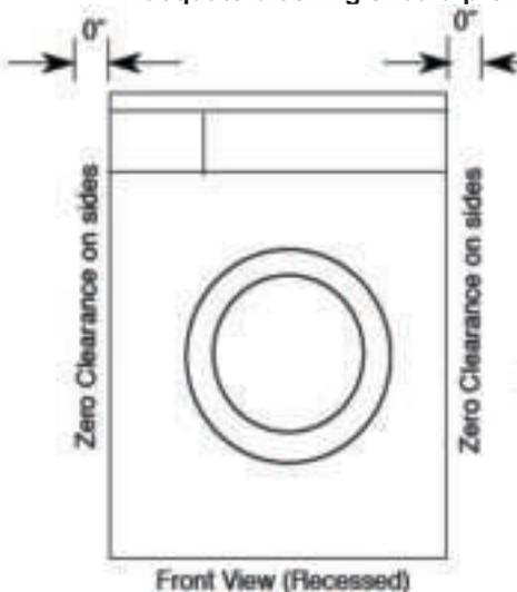
If the appliance is to be installed in a closet, the installation must be completed by a qualified person or service representative. Adequate blocking to secure unit is required. Additional clearances for floor, wall or door moldings may be required.
