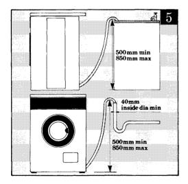
Finally, make sure that with the machine in position, the drain hose is not obstructed, blocked or bent so sharply that water cannot flow freely.
