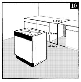
Having made the necessary electrical and plumbing connections as already described (see pages 8-11), you can now simply manoeuvre the machine into position. Take care, though, that in the process the fill and drain hoses are not kinked in such a way as to obstruct the flow of water, and ensure that you can still easily reach the power socket into which the machine is plugged.
