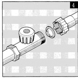
to fit the mesh filters supplied as per figure 4.
