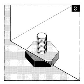
Some vibration is inevitable, especially if mounted on a wooden floor, so make sure there is a gap of at least 12mm ( $\frac{1}{2}$ ") between the machine and any walls, furniture and so on.
