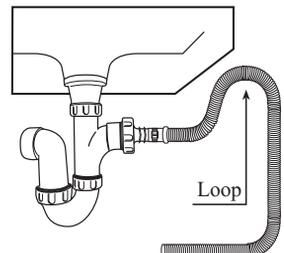
If you intend to drain the hose from the machine into a sink, make sure that the sink is empty and the plug hole is not blocked. Use the plastic "U -Piece" supplied.
