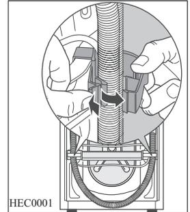
3. With the supplied spanner unscrew and remove the central rear bolt **A**.
