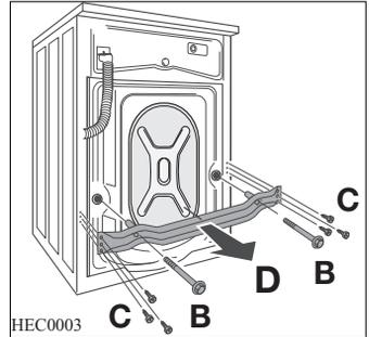
5. Remove the bracket **D** and refit the six smaller bolts **C**. Slide out the relevant plastic spacer **E**.
