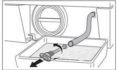
5. Release the emergency emptying hose, place it in the container and remove its cap.
