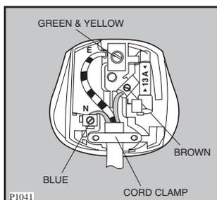
The wire coloured green and yellow must be connected to the terminal marked with the letter «E» or by the earth symbol  $\perp$  or coloured green and yellow.
