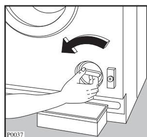
Unscrew and remove the filter.
