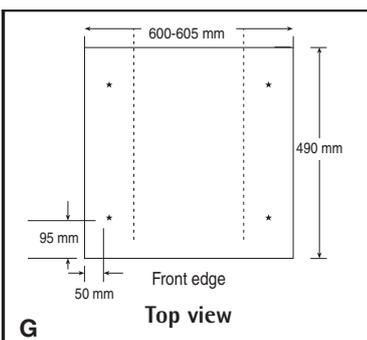
Position the base into the recess with its front edge as far forward as the adjoining plinth line will allow. **The reason for placing the base in this position is to allow a small strip of beading to be fitted in front of the appliance feet.**
