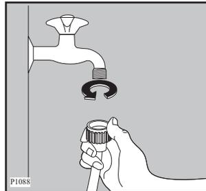
2. Set the hose correctly by loosening the ring nut. After positioning the inlet hose, be sure to tighten the ring nut again to prevent leaks.
