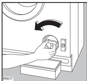
Unscrew and remove the filter.
