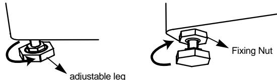
**③ Make it sure that the washer does not sway when you press down the four corners of the washer's top plate.**
