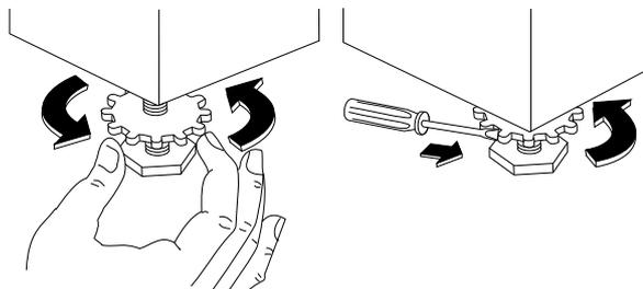
After having levelled the machine, tighten the lock nuts.
