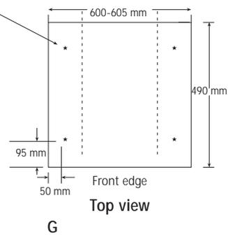
Fix the base firmly to the floor using four appropriate countersunk screws (see Fig. H).
