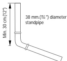
If you intend the drain hose from the machine to empty into a sink, make sure that the sink is empty and the plug hole is not blocked. Use the plastic "U -Piece" supplied.
