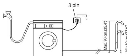
The upright standpipe should have a minimum length of 30 cm (12") from the bottom of the elbow to the top of the pipe (see diagram). Make sure that it is designed in such a way that the end of the drain hose cannot be covered with water.
