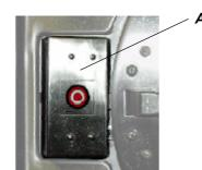
To open the door in case of emergency (malfunction, etc.), remove the lock cover plate (A). Subsequently,
