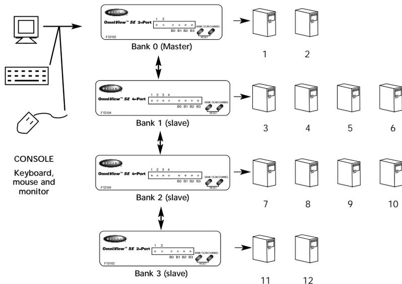
The OmniView™ SE has the capability to be daisy-chained to additional units for control over more computers. Up to four OmniView™ SE units can be daisy chained together, whether 2-Port, 4-Port, or a mixture of both. The example above shows two OmniView™ SE 2-Port units and two OmniView™ SE 4-Port units daisy-chained together.
