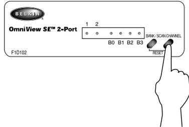
Pressing the CHANNEL button cycles you through all the ports, including inactive ports.
