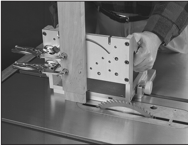
Figure 15. An example of vertical work: using the Shop Fox® for making tenons on the table saw.
