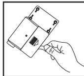
Remove the battery isolator
