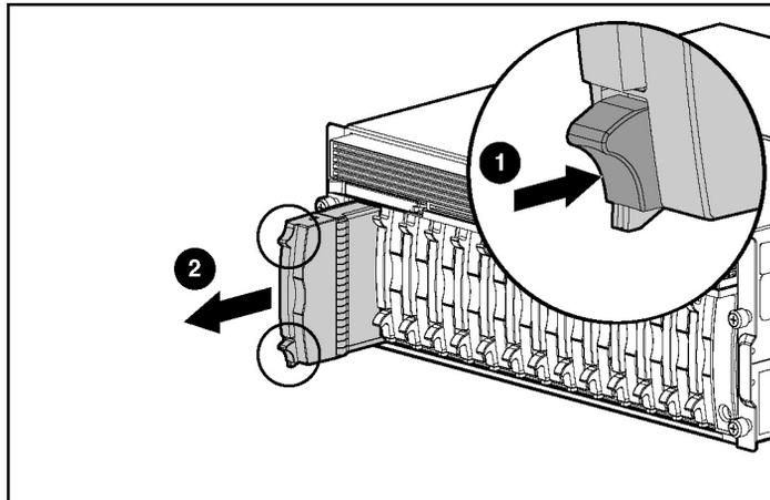
To replace the blank, slide the blank into the bay until it locks into place.
