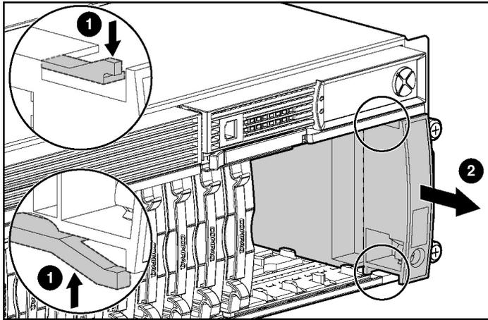
To replace the component, slide the power button/LED assembly into the bay until it locks into place.
