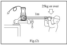
(c) How to Adjust the Position of Tool Holer;
