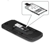
Note: If the card is not inserted correctly, the phone does not detect the SIM card. Remove the battery and re-orient the card back into the slot.
