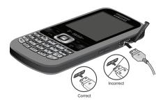
Note: The previous illustration displays the incorrect method for connecting the charger, If attempted, damage to the accessory port occurs therefore voiding the phone's warranty.
