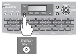
or Automatically enters the Power Saver Mode after 10 minutes (default setting) from the last operation.
