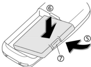
To remove, press the retaining tab ⑦ then lift the battery out.
