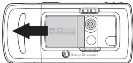
While in standby, slide the lens cover to activate the camera.
