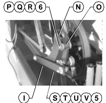
**CAUTION: BY REMOVING THE BOLT (V), YOU WILL BE SEPARATING THE PEDAL LEVER ASSEMBLY AND THE 14" LINK BAR ( I ), THIS WILL CAUSE THE CRANK ARM ASSEMBLY TO ROTATE.**
