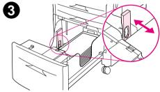
Adjust the front (X) paper guide by squeezing the tab on the guide and sliding it to the edge of the paper.
