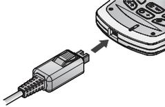
When charging is complete switch off the mains power supply and disconnect the charger by pressing the button on the connector ❶ and remove from the base of the phone ❷.
