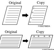
• When making copies from either the A3L or B4L size, the copier autmatically speify the hole punching position as shown below.
