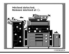
If a paper misfeed occurs during a copy cycle, the message shown on the left appears and that particular copy cycle is stopped in the middle of operation.
