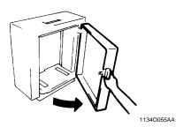
When adding paper to a partially loaded Cassette, press the Paper Plate Descent Key to lower the Paper Plate before opening the Cassette Door.
