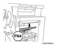
Remove the sheet of paper and close Misfeed Clearing Guide **FN4**.
