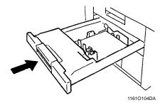
Slide the Edge Guides in the direction of the arrow to suit the paper size.
