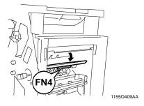
Remove the sheet of paper and close Misfeed Clearing Guide **FN4**.
