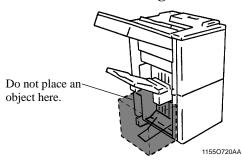
NEVER place an object under the Bottom Offset Tray or Elevator Tray. Anything that is placed under the Bottom Offset Tray or Elevator Tray can interfere with the tray when it lowers after a copy set has been fed onto it, which results in a malfunction.
