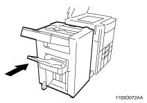
9 Touch **Staple** and the copier automatically feeds a sheet of paper to test the stapling.
