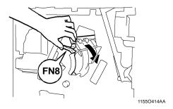
Remove the sheet of paper and close FN8 .
