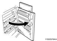
7 Turning Knob  $\boxed{\text{M2}}$ , pull out the sheet of paper.
