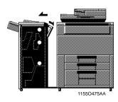
**1** Holding the Finisher Lock Release Lever, slide the Finisher away from the copier.
