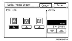
Hold down the 🔻 or 🔺 key until the desired erase width is reached.
