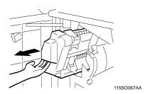
While pressing down the Staple Cartridge Lever, pull the Staple Cartridge out its port.
