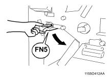
Remove the sheet of paper and close **FN5**.
