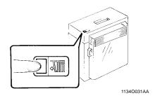
2 Holding the Door Lock Release Lever, open the Cassette Door and remove the sheet of paper.
