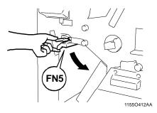
Remove the sheet of paper and close **FN5** *16*
