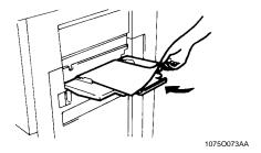
To reset the paper misfeed indication on the Touch Panel, open and close the Front Door.
