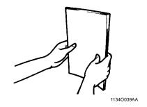
3 Insert a neat stack of papers face down into the Staple Tray.
