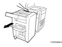
2 Opening Misfeed Clearing Guide FN1 remove the sheet of paper.
