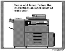
When toner has run out, the message shown on the left appears and you can no longer start a new copy cycle. Replace the Toner Bottle with a new one by following the procedure given below.
