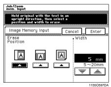
8 Using the or key, set the desired erase width.
