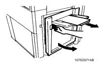
Pull out the sheet of paper from the Paper Take-Up Section. Then, close the Right Door.
