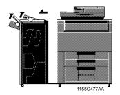
Open Exit Tray **FN9** and remove the 1 sheet of paper.
