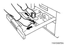
Load the paper stack into the Drawer so that 3 its front side faces down.
