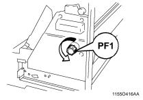
11 Check to see if a sheet of paper is left in the Finisher. If any is visible, perform step 10 once again.
