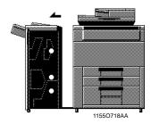
Holding the Finisher Lock Release Lever, 1 slide the Finisher away from the copier.
