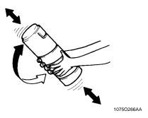
With the "UP" marking on top, insert the Bottle into position.
