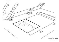
**3** Position the original in the left rear corner with the ↑ marker on the scale.
