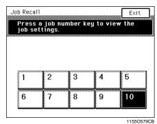
3 Check the settings made and then touch **Exit** . The copier is set up for these settings and the Basics screen reappears.
