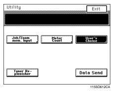
Select the key of the page number on which 3 the desired User's Choice function is listed. For example, to change Output Priority from Non-Sort to Sort, touch 2/6
