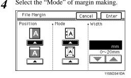
5 Hold down the ▼ or ▲ key until the desired margin width is reached.
