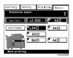
When the drawer currently selected for use runs out of paper, the message shown on the left appears. The current copy cycle is interrupted and you cannot start a new copy cycle. The blinking drawer has run out of paper.
