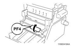
Turning Knob **PF1**, remove the sheet of 20 paper and then lower Misfeed Clearing Guide **PF4**
