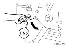
P Remove the sheet of paper and close FN5.
