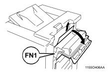
**3** Loosen two screws, open the Misfeed Clearing Guide and remove the sheet of paper.
