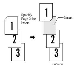
The copier inserts a blank sheet of paper for inserts (e.g., color paper) at any specified place between pages.
