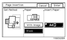
Select the paper source in which paper for inserts has been loaded in step 5.
