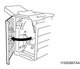
Raising Misfeed Clearing Guide FN3, remove the sheet of paper.
