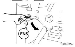
Remove the sheet of paper and close  $\boxed{\textbf{FN5}}$ .
