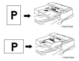
• If you need to load your original in a direction different from these examples, set the direction of the original on the Touch Panel. \*p. 3-37
