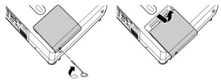
6. Use the screwdriver to loosen the two screws holding the lamp in place. You can't remove them.
