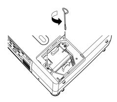
8. Hold the lamp as shown and pull it straight out.
