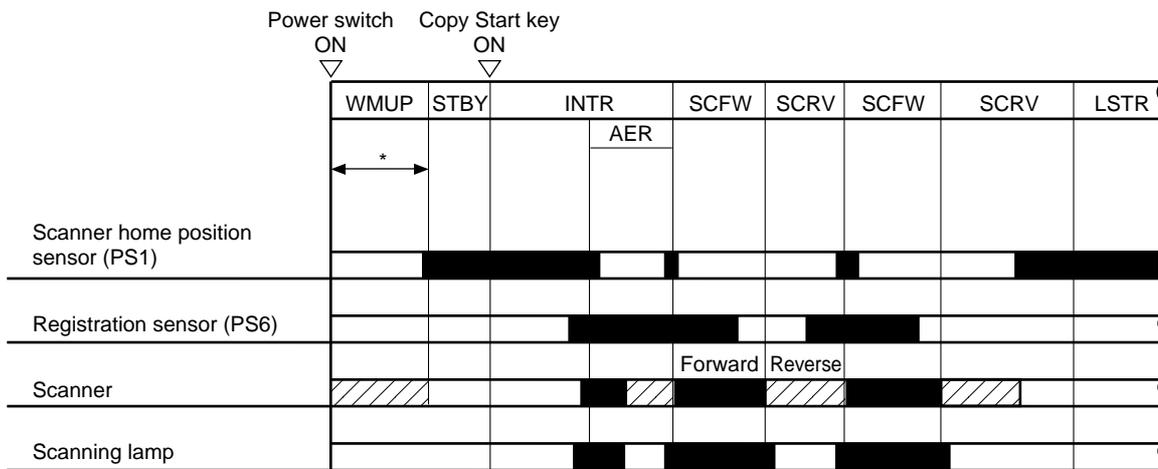
\*The scanner is returned to home position at power-on whenever the scanner is not at home position.
