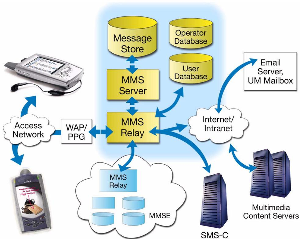
Figure 3. The architecture of MMS
