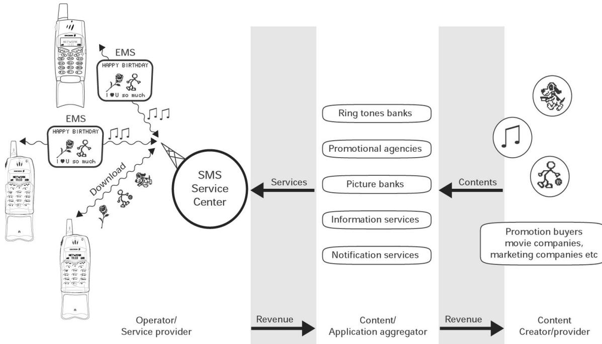
The diagram shows a model over the possibilities with Enhanced Messaging Service:
