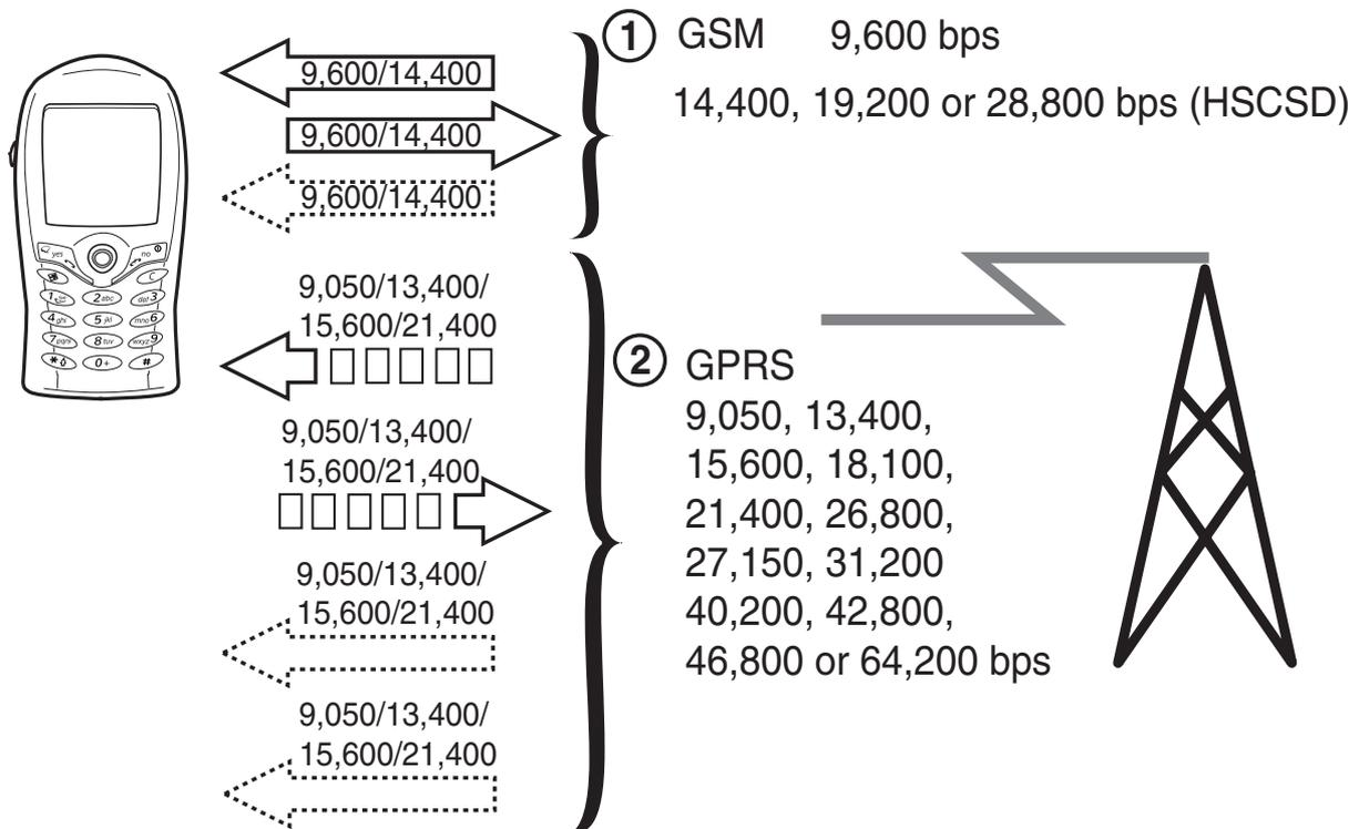
Figure 4 A comparison between GSM and GPRS
