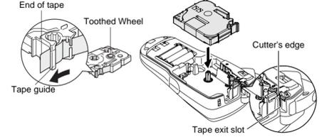
Make sure that the end of the tape feeds under the tape guides. If the ink ribbon is loose, use your finger to wind the toothed wheel in the direction of the arrow on the cassette. Use only Brother TZ tapes with this machine.
