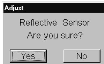
3. Click on the **Yes** button and the sensitivity of the reflective sensor will automatically be set as indicated by the "Now Adjusting" window appearing as shown in the figure below.
