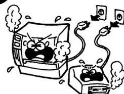
Continued use of the machines in an abnormal condition such as when the machines are producing smoke or strange smells may cause **fire** or **electric shock**. In these cases, immediately turn off the power switches and disconnect the power cord plugs from the outlet. Then, contact your authorized TOSHIBA TEC representative for assistance.
