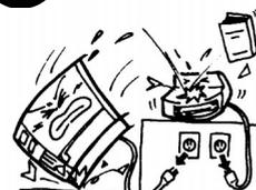
If the machines are dropped or their cabinets damaged, first turn off the power switches and disconnect the power cord plugs from the outlet, and then contact your authorized TOSHIBA TEC representative for assistance. Continued use of the machine in that condition may cause **fire** or **electric shock**.
