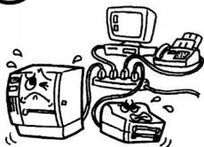
If the machines share the same outlet with any other electrical appliances which consume large amounts of power, the voltage will fluctuate widely each time these appliances operate. Be sure to provide an exclusive outlet for the machine as this may cause **fire** or **electric shock**.
