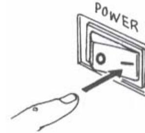
When the power switch is switched on, initial startup message [Manual Print Mode] is displayed on the touch screen.
