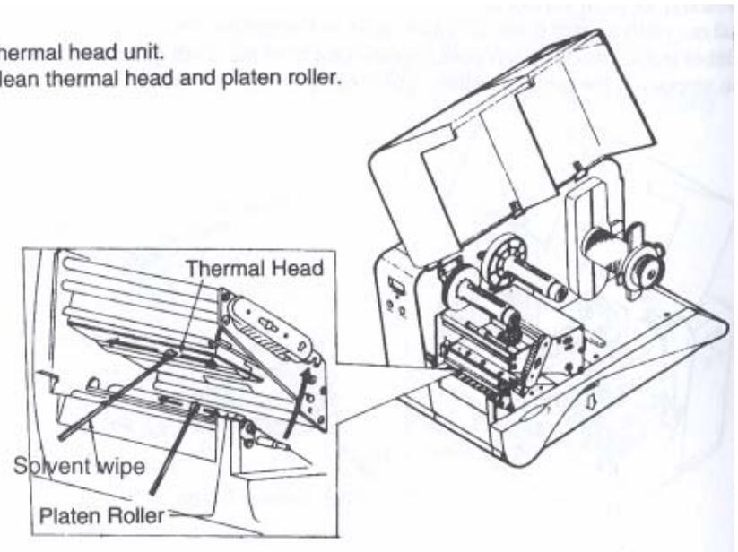
Cleaning method for printer parts
