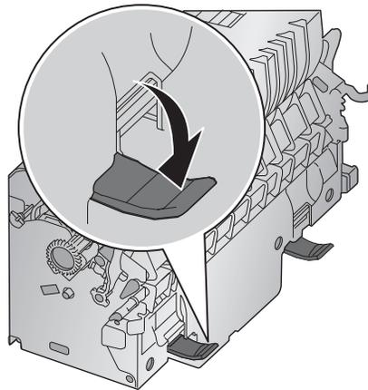
4. Pull the fuser out, and set it on a clean, flat surface.
