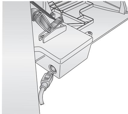
17. Remove the packing tape from the rewinder **dancer arm** and move it into the up (starting) position.
