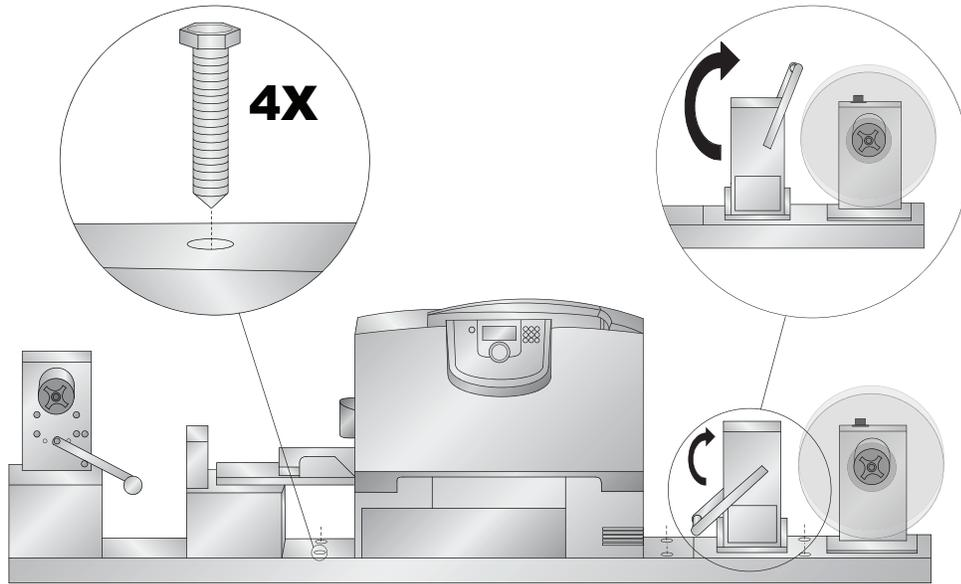
**Warning:** To prevent serious injury you must bolt the CX1200 to a table or bench. Use the included lag bolts and predrilled holes in the base.
