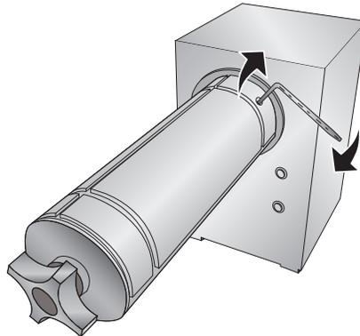
6. Locate the rewriter (right side) chuck and the label guide disc with the three interior holes. Attach the label guide disc to the rewriter (right side) chuck using two flat head bolts provided.
