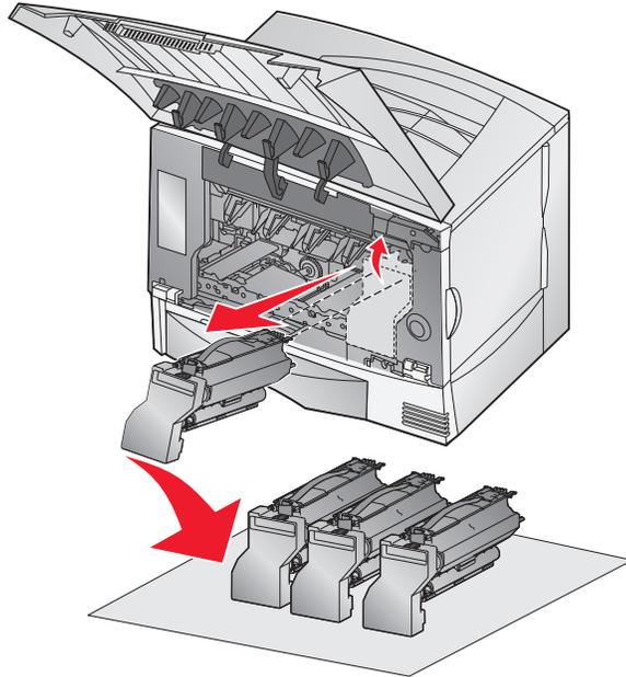
Before replacing the toner cartridges, shake the cartridges side to side and back to front to redistribute toner. Next, remove the protective sheet from the bottom of each toner cartridge. Put cartridge(s) back into the printer being sure to match the color label on the cartridge with the one on the printer. On each cartridge there are pegs that correspond to slide rails inside the printer.
