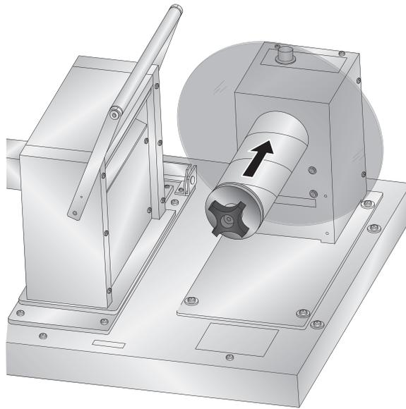
6. Place the outer label guide disc on to the rewinder chuck. Push the guide until it touches the rewinder core. Turn the tension knob clockwise to secure the core and the label guide to the chuck.
