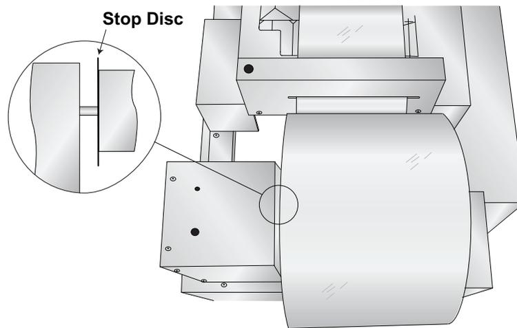
**Note:** You must use only 8.5 inch wide label stock in the CX1200. Failure to use specified label stock will result in damage to your printer and excessive build up of toner and adhesive inside the printer.
