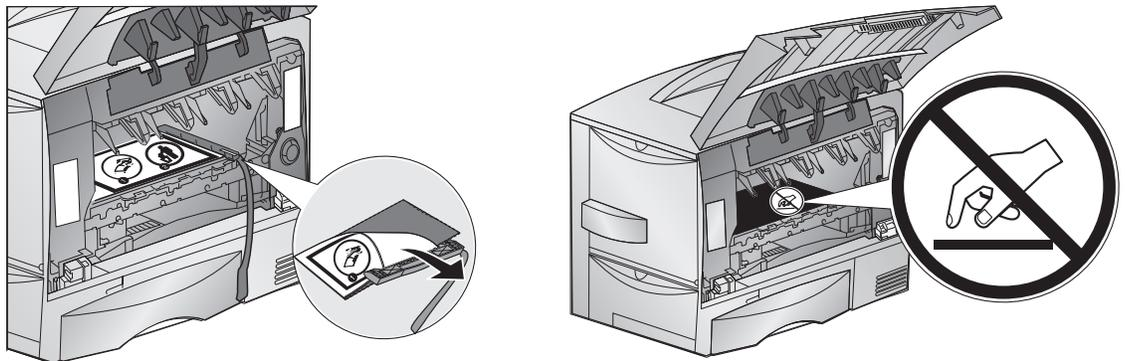
13. Before replacing the toner cartridges remove the red plastic protection plate from the bottom of each toner cartridge. Put cartridges back in to the printer. On each cartridge there are pegs that correspond to slide rails inside the printer.
