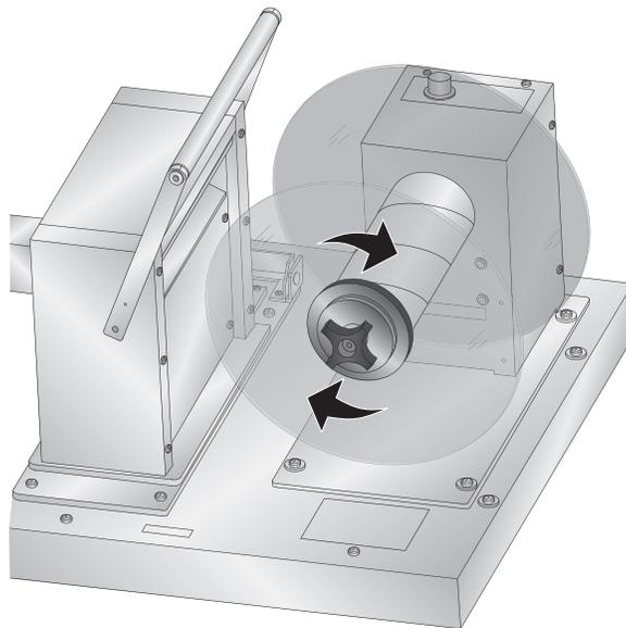
**Note:** Some cores may be shorter than the the stock width. If so, make sure the distance between the label guide discs is slightly larger than the stock width.
