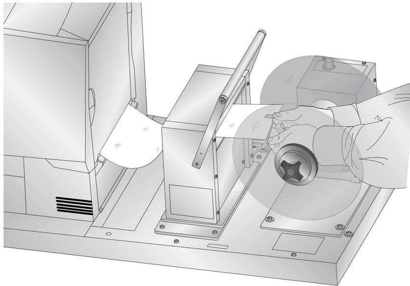
**Note:** Make sure the stock feeds under the rollers inside the tensioning unit. If possible use your left hand to guide the stock under the roller as it exits the printer.
