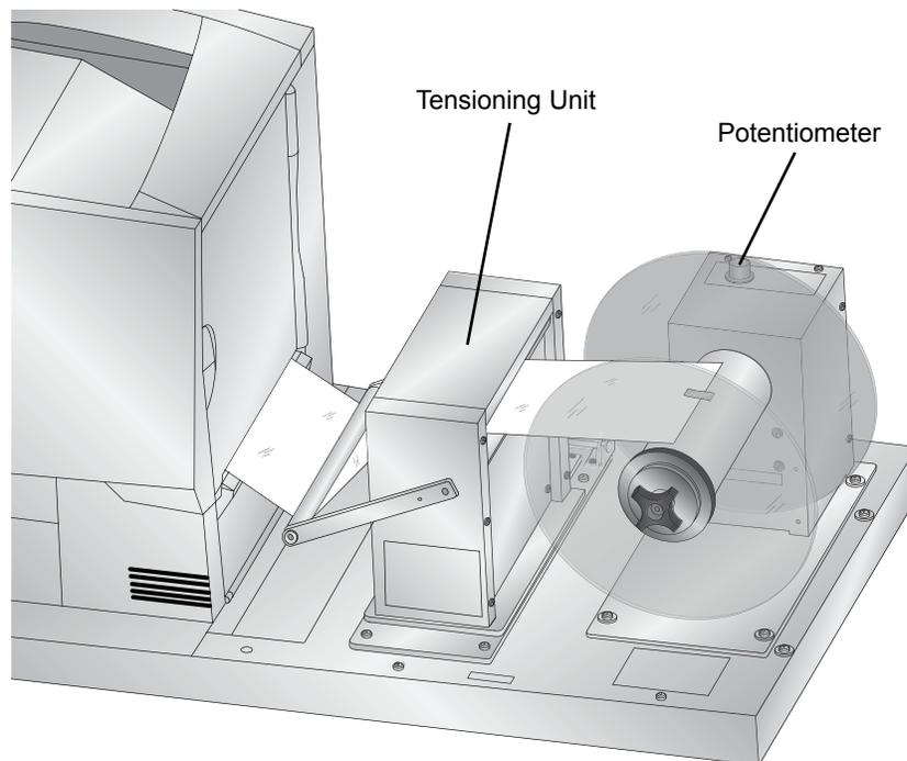
**Note:** Use the **Potentiometer** on the top of the rewinder to increase or decrease tension to get a tighter or looser wrap. If the stock is slipping through the clamp in the tensioning unit, you may need to decrease the tension.
