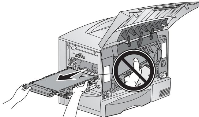
4. Insert a new image transfer unit back into the printer.
