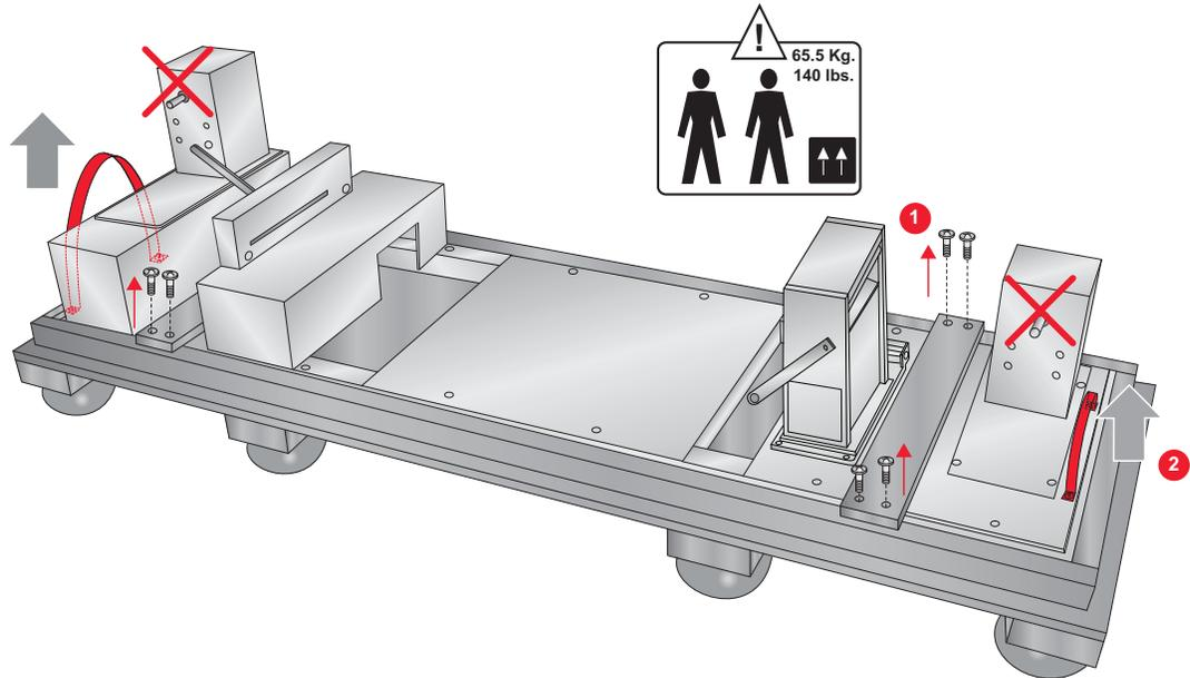
Now remove two screws and washers from each side to remove the nylon handles. Finally, replace the screws only.
