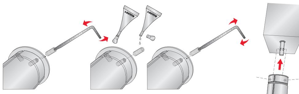
5. Tighten the set screws using the 3mm allen wrench. Once they are tight, attempt to rotate the chuck forward backward while watching the drive shaft. The drive shaft should move with the chuck. If it does not move with the chuck, loosen the set screws slightly and turn the chuck until the set screws are even with the flats. The Loctite will dry in 24 hours.
