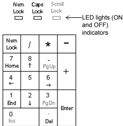
Figure 3-5. The numeric keypad and LED indicators.
