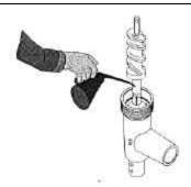
The shaft of the feed screw should be lubricated with grease before the feed screw is inserted into the housing. Use e.g. paraffin oil or castor oil, never salad oil.
