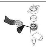
The thread of the housing should be lubricated with grease before the distance ring and the ring are mounted. Use e.g. paraffin oil or castor oil, never salad oil.
