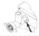
When the meat mincer has been assembled, it is mounted in the attachment engagement hub of the mixer. The meatmincer must be pressed into the attachment engagement hub before the thumb screw is tightened.
