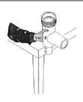
Place the housing on the edge of a table, the opening upwards, when the meat mincer is to be assembled.
