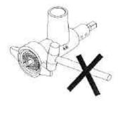
The ring should only be screwed slightly on by hand.
