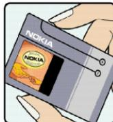
2. When you angle the hologram left, right, down, and up, you should see 1, 2, 3, and 4 dots on each side respectively.
