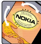
3. Scratch the side of the label to reveal a 20-digit code, for example, 12345678919876543210. Turn the battery so that the numbers are facing upwards. The 20-digit code reads starting from the number at the top row followed by the bottom row.
